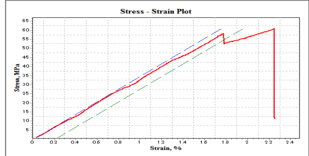
Fig 7: Experimental Flexural Stress-Strain Curve
